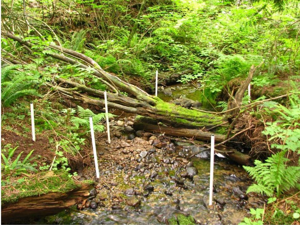
**Figure 3.9 Piezometer network across and around a meander bend in reach UA.**
